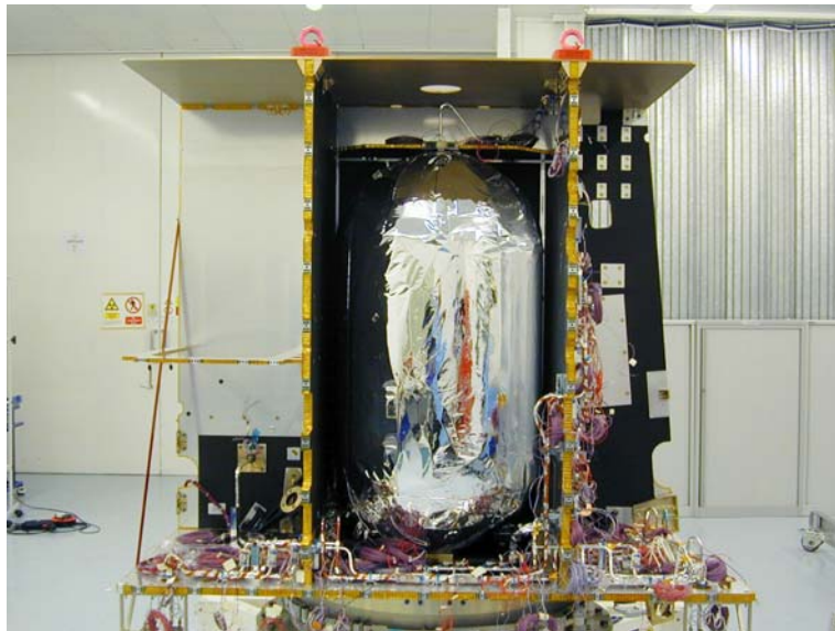
Figure 2. MeX propulsion system and mechanical structure
